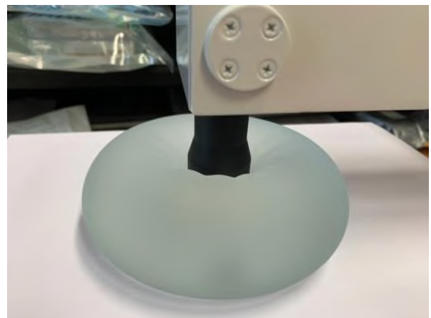
Fig. 1: Indentation test of breast implant.
