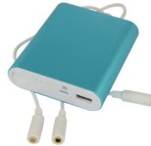
Fig. 6: Last version of designed device Wearable Telehealth Multi-Sensor Monitor (WTMSM) with ECG, RR and SCR sensors.
