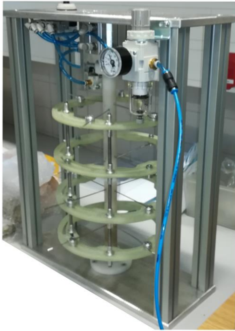
Fig. 5: Cyclic testing device assembled with a composite external fixator
