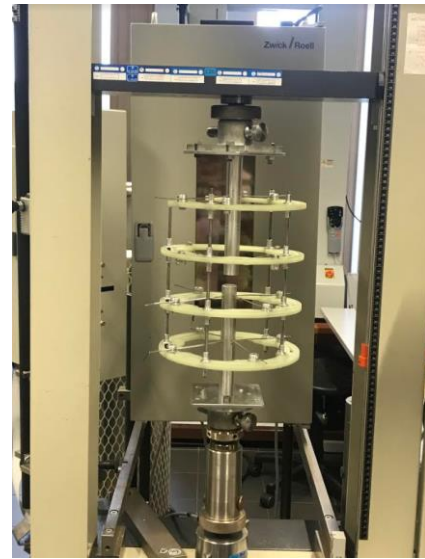
Fig. 4: Pressure test assembly
