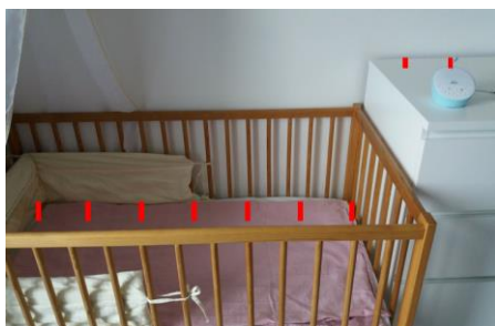
Fig. 1: Measurement setup around the electronic baby monitor (red stripes indicate the points where measurement is performed).
