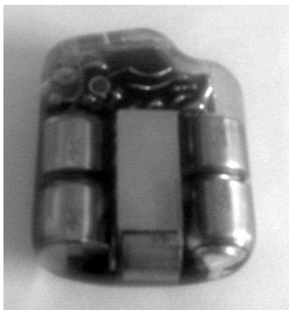
Fig. 2. Pacemaker VVI (on demand) from 1968 with epoxy resin case
