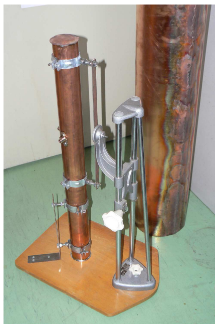
Fig. 4. Applicators for 2.45 GHz (smaller) and 915 MHz (bigger)
