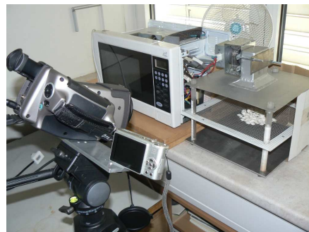
Fig. 1. System for visualization of microwave exposure of various materials
