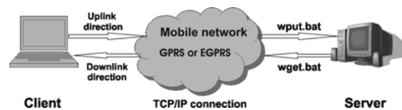
Fig. 2. General measurement description
