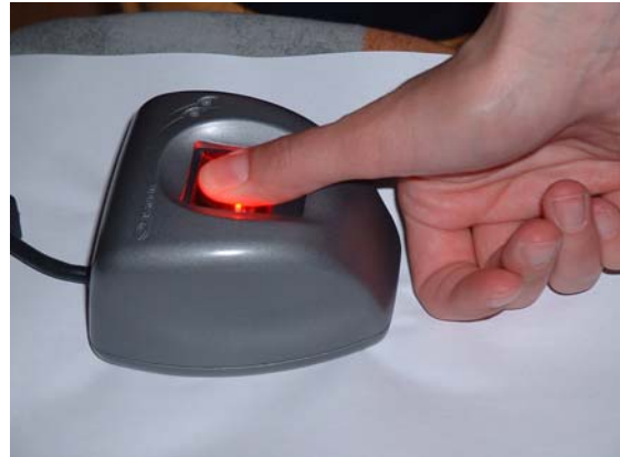
Fig. 3 Fingerprint nail-to-nail pattern scanning (optical Sagem Morpho sensor)
