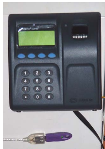
Fig. 4 Biometrics fingerprint control hardware - identification device (MA) and dongle (below)
