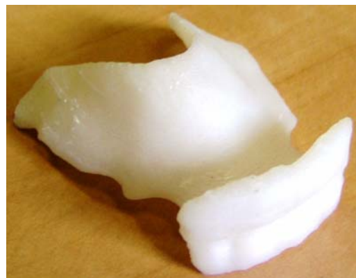
Fig. 4 Real 3D model of partial denture produced by SFF machine using FDM technology and ABS material
