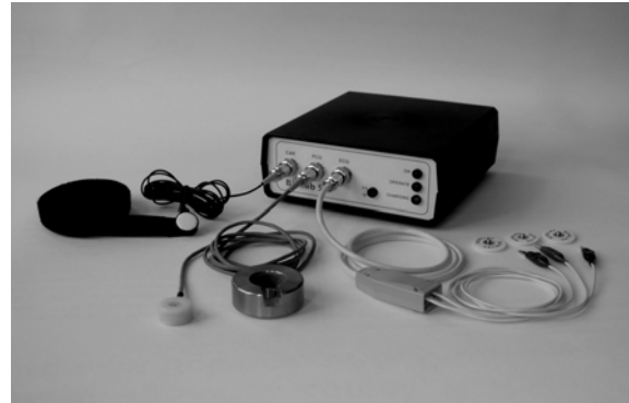
Fig. 3. BioLab STI smart sensor module with ECG electrodes, cardio microphone and piezzo-electric sensor of the carotid pulse wave.
