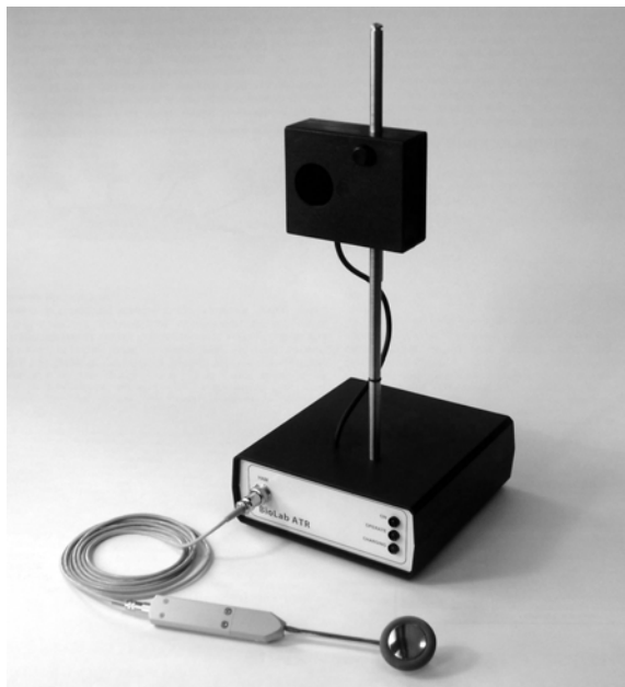
Fig. 2. BioLab ATR smart sensor module with optoelectronic sole movement sensor and synchronized stimulating neurological hammer.
