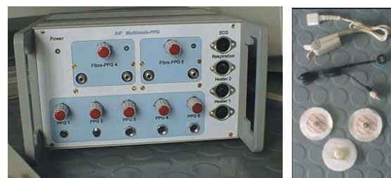
Fig. 1. Multi sensor measuring system capable of simultaneously reading multiple PPG channels, ECG and breathing signals.
