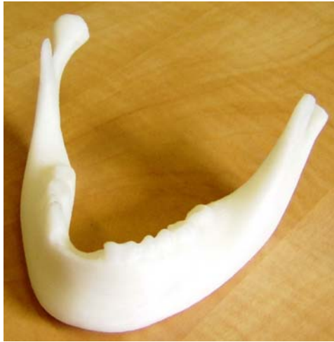
Fig. 8 Real 3D model based on CT data produced by RP machine
