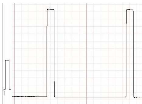
Pic. 4: The 300 \mu V response of ECG recorder, lead I, low frequency cut off: < 0.01 Hz, 20 mm/mV, good fulfilment of requirements
