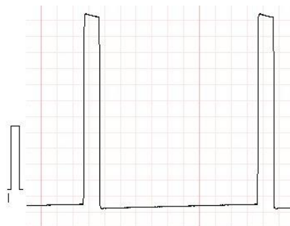
Pic. 5: The 300 \mu V response of ECG recorder, lead I, low frequency cut off: 0.05 Hz, 20 mm/mV, good fulfilment of requirements
